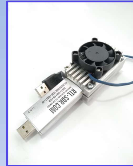
Heat dissipation system powered by USB
