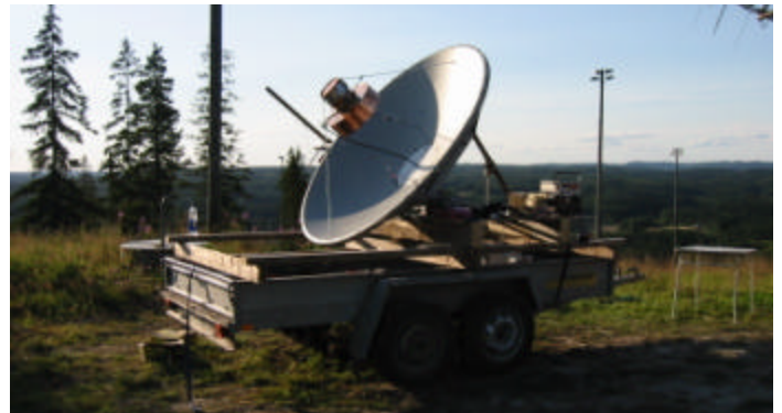
OH1FF/p Field Day station – 1.8 m dish and 50 W
