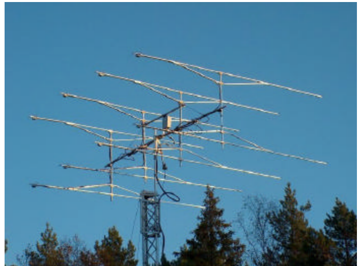
SM5IOT's new 12 x 25 el yagi array - Look for Chris on 70 cm in Nov
