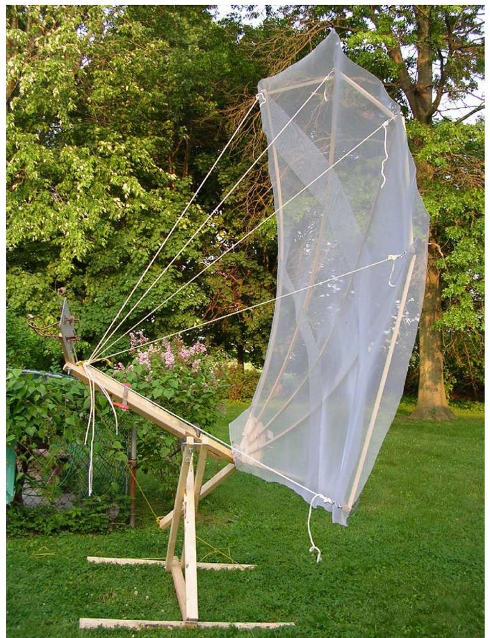
**7.5' offset stress dish for portable operation**
