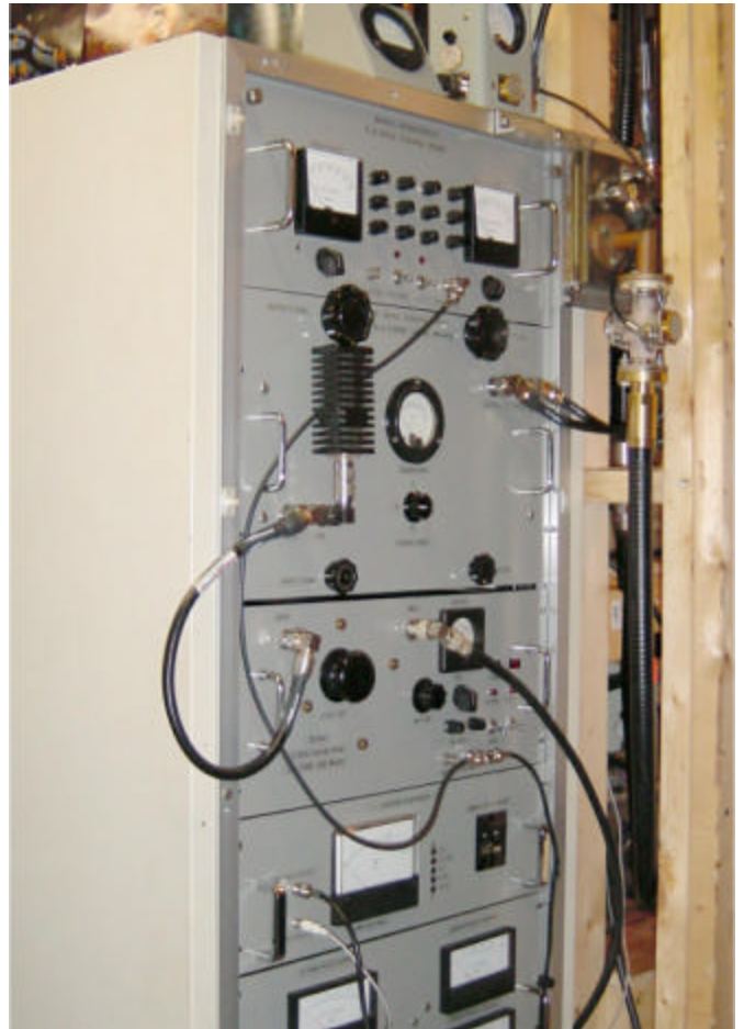
W4SM's completed dual 6 x 7289 ring 1.4 kW K2AH PA
