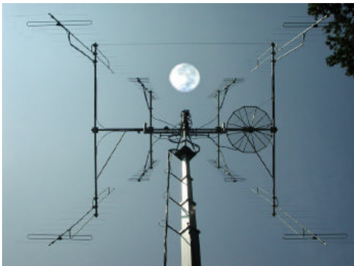
DL7UAE's antennas – 70 cm 4 yagi array is in the center
