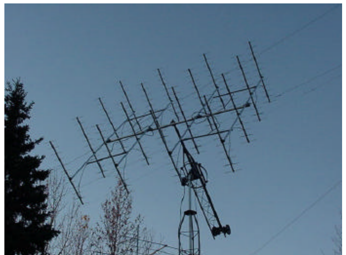
KL7FH's 16 x 12 el 70 cm array with full el and pol rotation
