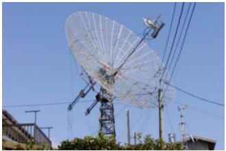
JA6XED's new 8 m dish with feeds for 70 and 23 cm
