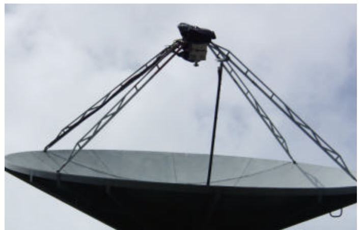
OK1KIR's dish with the 6 cm feed in place
