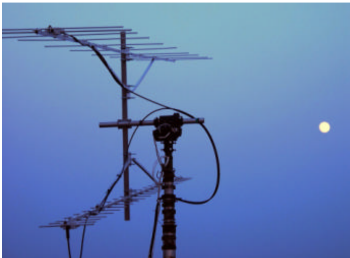
OK1TEH's 70 cm 23 el 18 dBi yagi below his 2 m yagi
