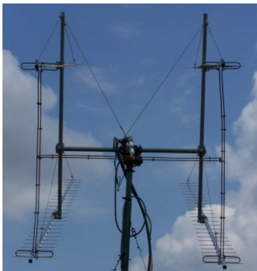
SP7DCS's 4 x 25 el I0JXX yagis with open wire feed system
