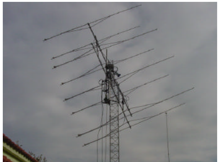
SV1BTR 8 x 39 el 13 wl yagi array used to complete WAC
