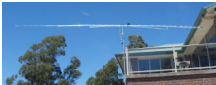
VK7MO's 35 el yagi and balcony location
