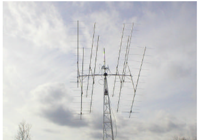
K5GMX's array of 4x25 FO yagis on 432 inside the 4x13 13b2 2 m yagis. Bill is QRV and interested in skeds connerwa@comcast.net
