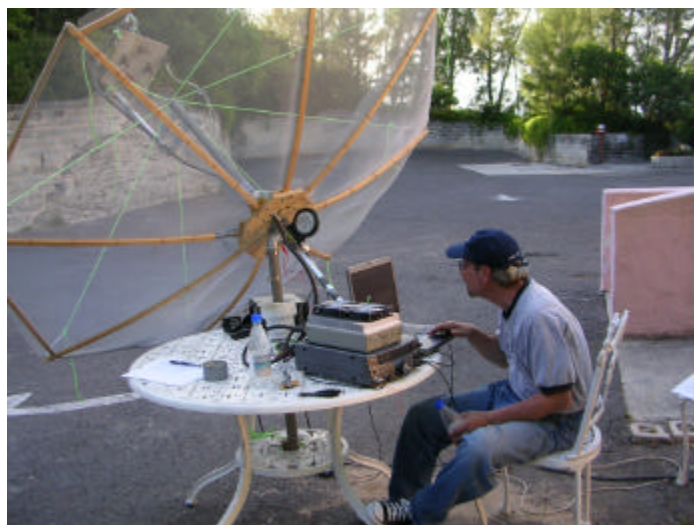
VP9/K2UYH with 7' stress dish and quad dipole circular feed
