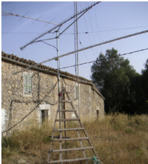
EA6VQ's single yagi used on 70 cm EME (1296 in the future?)
