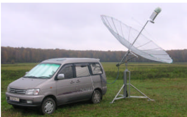
UA3DJG/UA3ATS' 23 cm portable EME station with 3 m stress dish
