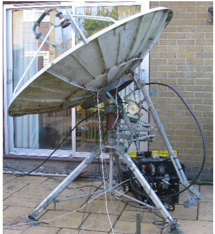
GM4ISM's 1.8 m dish used to work 8N1EME on 5.7 GHz
