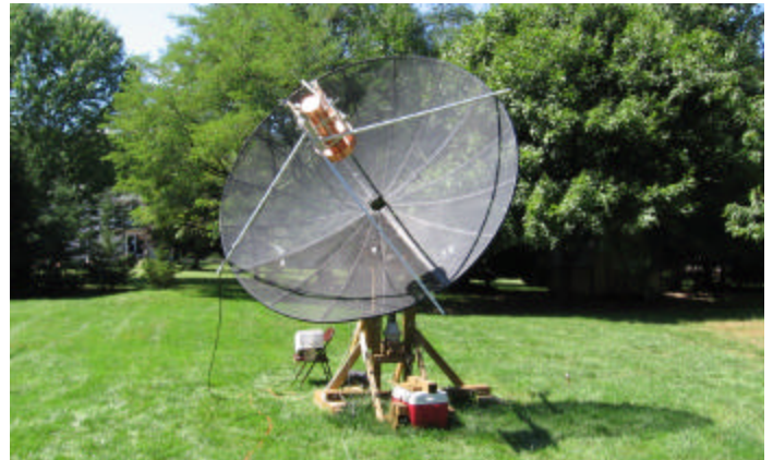
WA8RJF's 10' dish and 1295 test location
