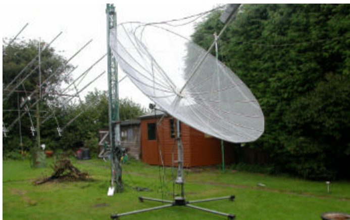
G4RGK's relocated 3.5 m stress dish with 432 array to side
