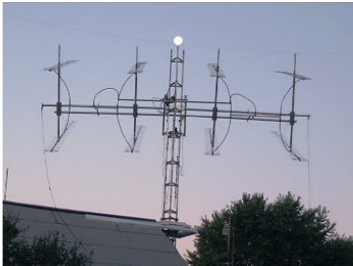
W8TXT new 8 FO-24 yagi array for 70 cm
