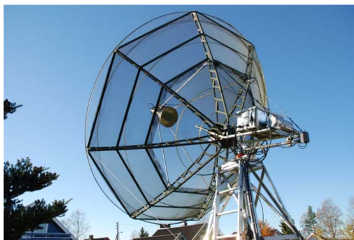
LA5ZK's 3.7 m dish for 1296 with PA mounted at the rear
