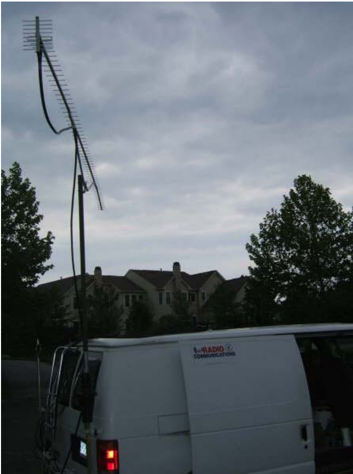
K1DS set up for portable 1296 EME using a WIMO1 yagi
