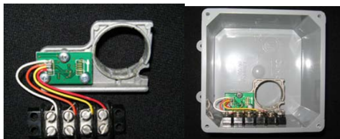
Fig 3. Accelerometer, pigtail & term strip mounted in weatherproof box
