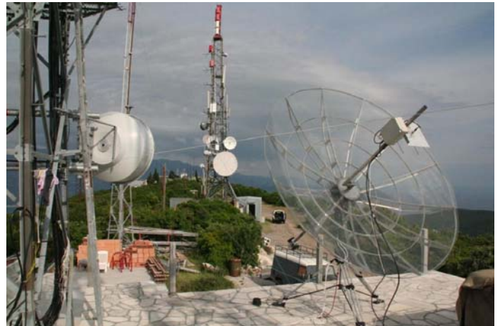
40/OK1DFC 3.2 m dish with 432 feed
