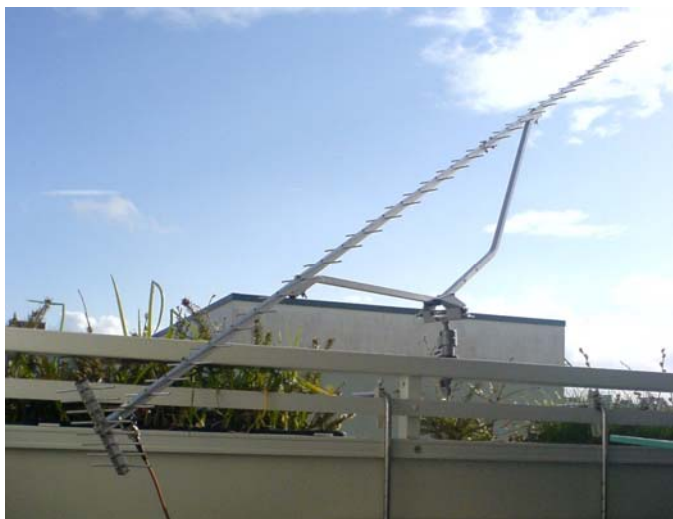
DJ8MS's long 67 el yagi used on 1296 EME
