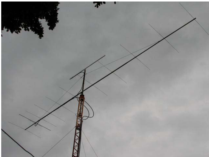
LY2BAW's 45 el loop yagis & 50 W used for 23 cm 1st EME
