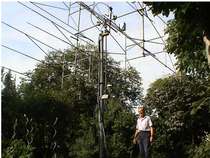
DL9KR 70 cm DXCC #1 with his 16 x long yagi array
