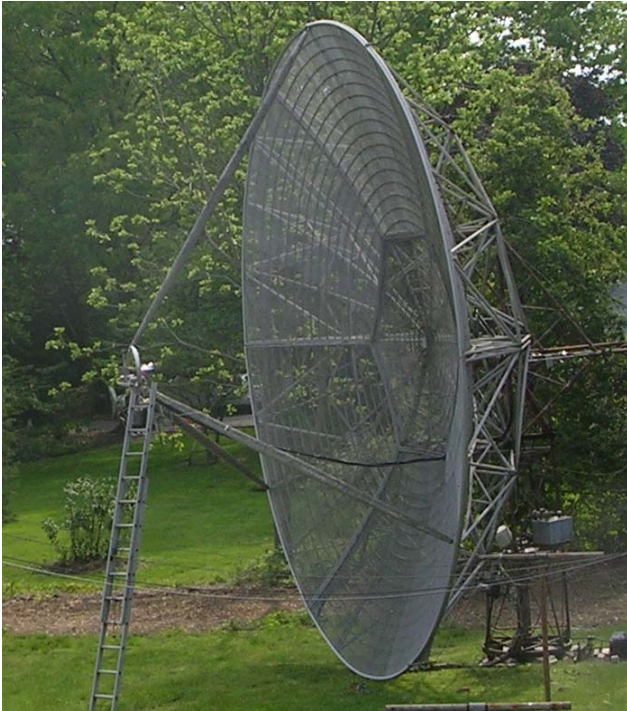
K2UYH's 28' dish with 1296 horn and off set 432 feeds
