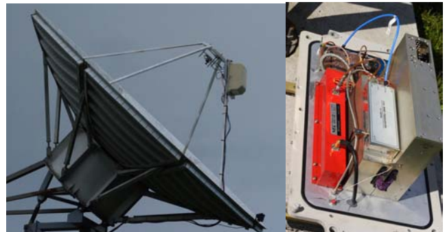
ES5PC dish with the 10 GHz feed box shown on the left
