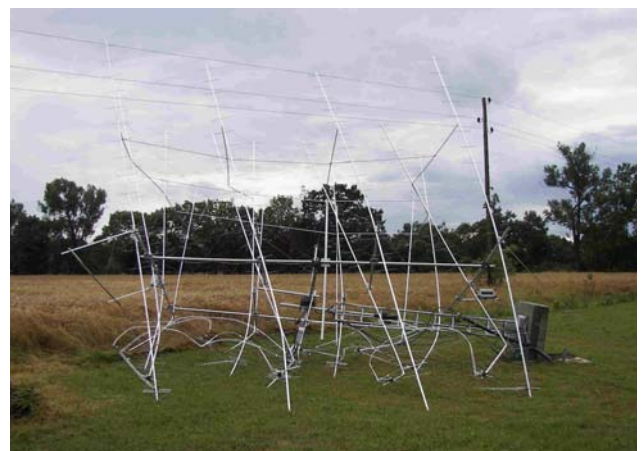
DL7APV's 432 array after the storm!
