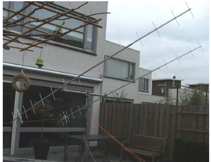
PE1RDP's 2 yagi array for 70 cm EME
