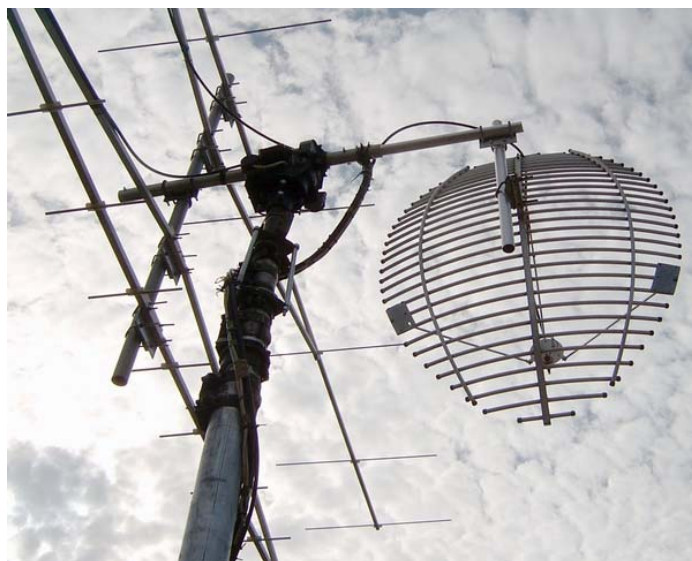
OK1TEH's antennas including dish used on 23 cm EME
