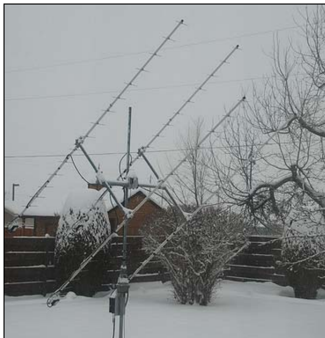
KA7V's 4 x CC 5.8 wl yagis array for 70 cm EME from OR
