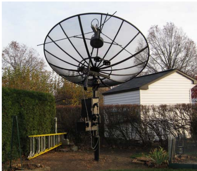
W3HMS' 3 m dish with 1296 feed
