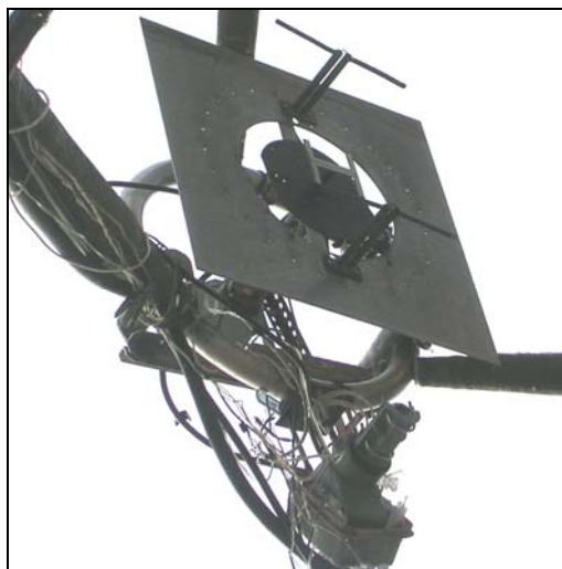
K2UYH's rotatable linear feed for 70 cm (hor) & 23 cm (vert)
