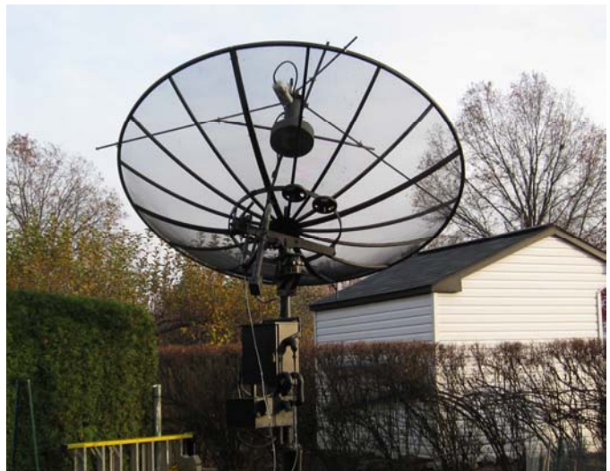
W3HMS 10' TVRO dish used on 1296 EME
