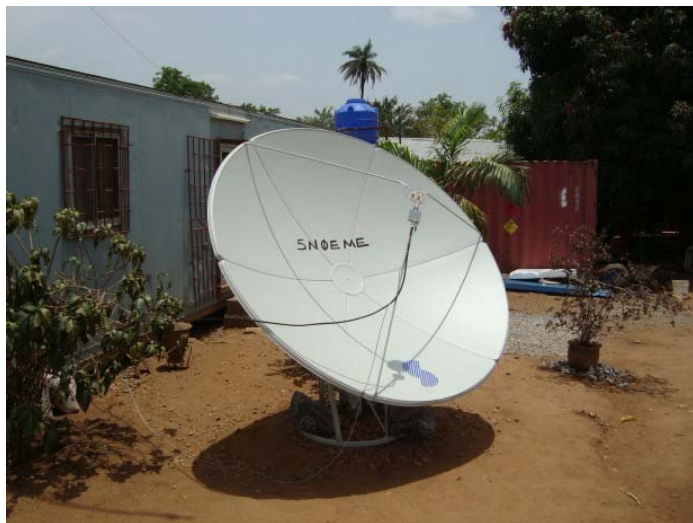
5N0EME 2.4 m dish used on 23 cm
