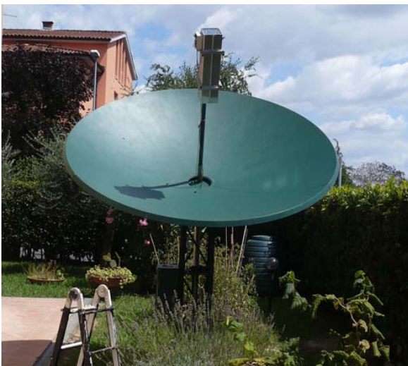
IK5OLO's 2.4 m dish with septum feed for 23 cm
