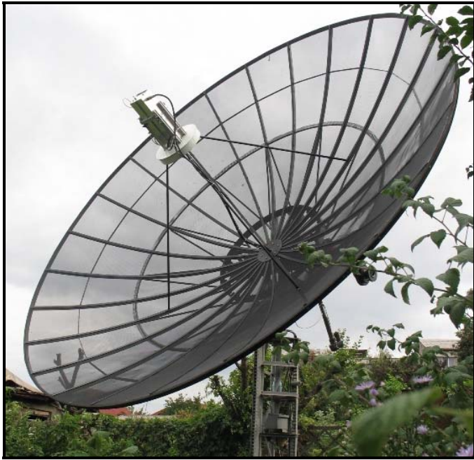
YO8BCF's 4.9 m dish with OM6A multi-ring feed
