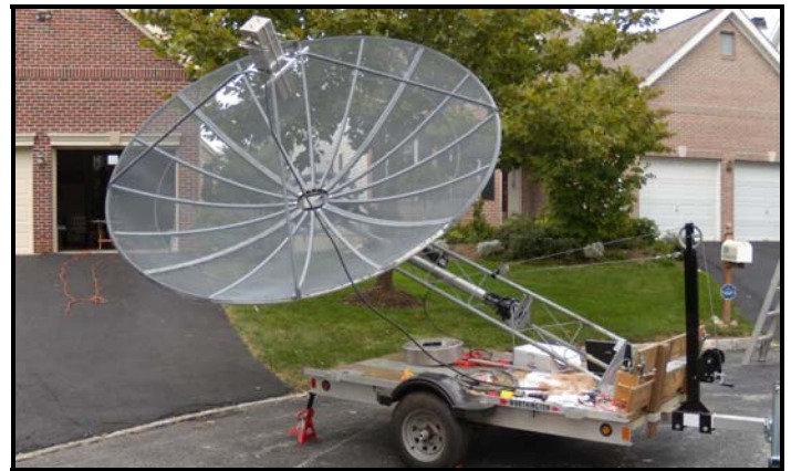
K1RS's new portable EME system under test. Look for Rick on 1296 EME soon.
