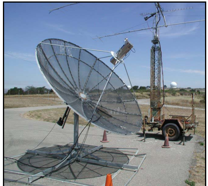
N6VMO is QRV on 23 cm with 10' TVRO dish and 300 W
