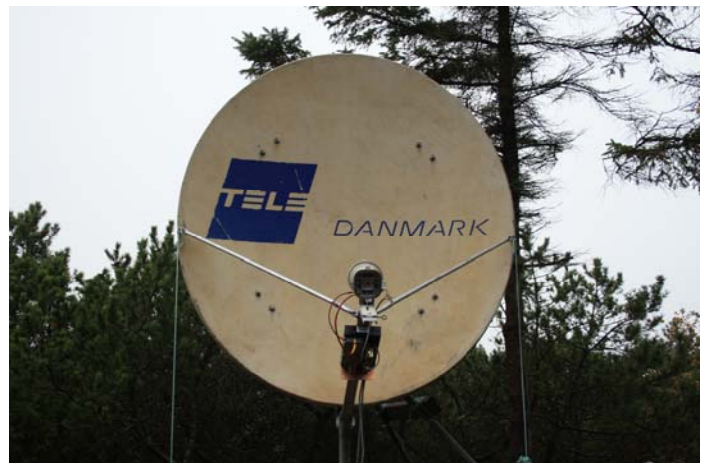
OZ1IFF's 1.8 m dish used successfully on 10 GHz
