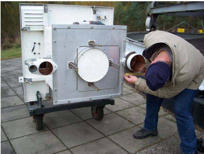
PI9CAM feed box with 3, 6 and 13 cm feeds in place with PA3CEG adjusting the 13 cm feed – see report later in NL.
