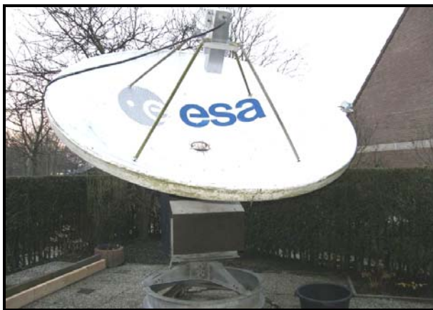
PA0PLY's 1296 3 m dish used with a100 W SSPA.
