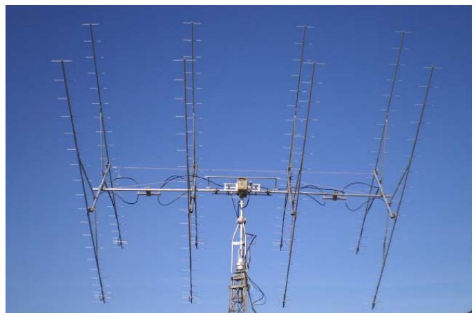
G4DHF's 8 x 21e1e refurbished Tonna Array for 70 cm
