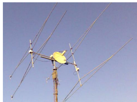
S57SU's 1.2 m dish for 23 cm EME in middle of 2 m EME array
