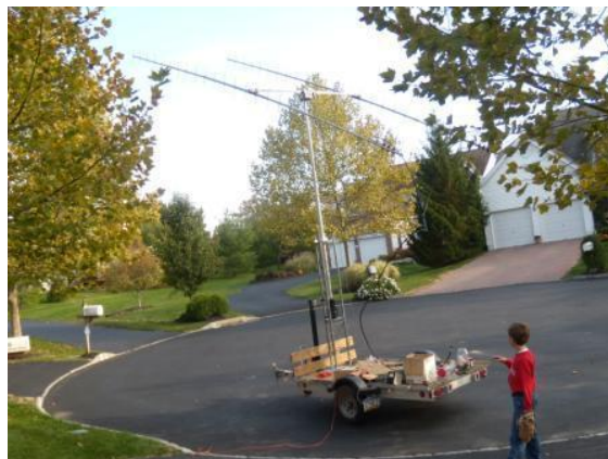
KIDS' portable 70 cm EME antenna system
