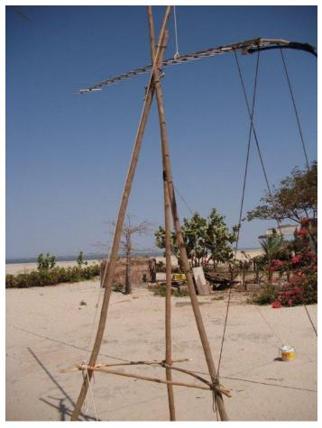
C56EME yagi and locally constructed mount in Gambia
