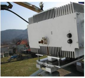
OK1KIR is back on 24 GHz EME after 3 years break – new 24 GHz TX/RX (23 W SSPA) box is rotatable at the dish focus.
