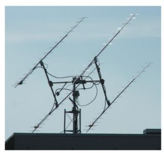
PE1RDP's new 4 x DK7ZB yagi array
