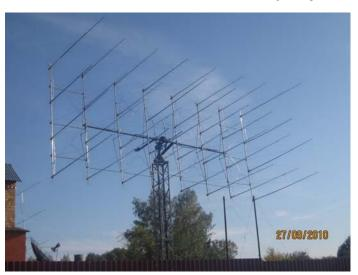
UA3PTW's 24 yagi array used on 70 cm (23 cm dish lower left)
