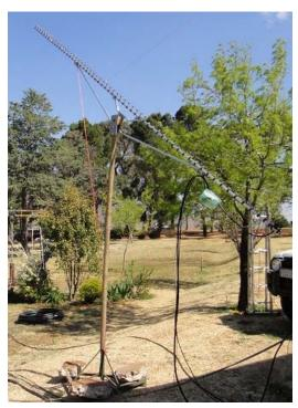
7P8HP 23 cm 62 el yagi used with 400 W SSPA
