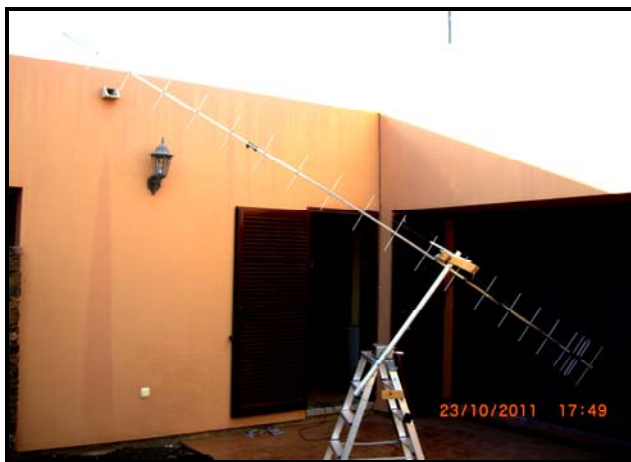
EA8/G4RGK's antenna arrangement for 70 cm EME
