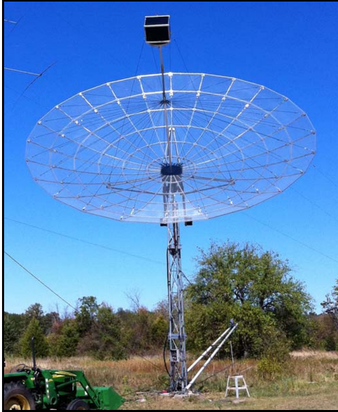
K5GW's new 32' stress style dish for 70 cm EME
