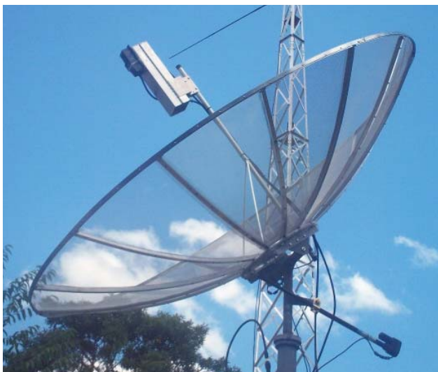
PY1UNU's 3.36 m dish with 1296 septum feed
