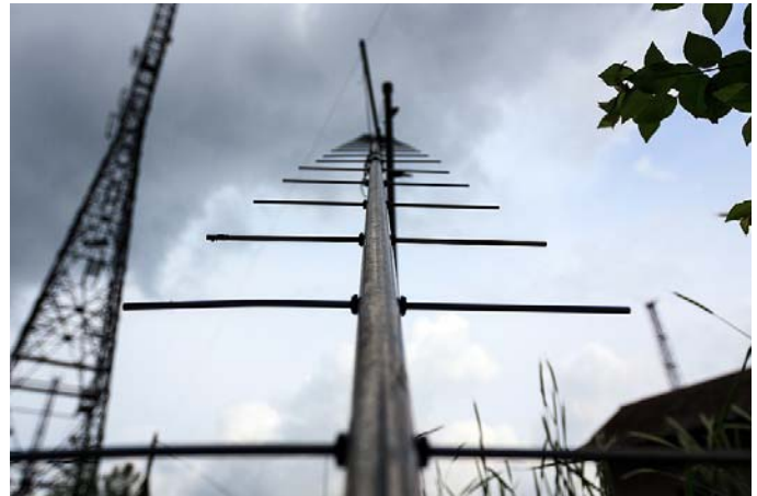
38 el M2 yagi at EY8ZF (left there for future 70 cm EME)
