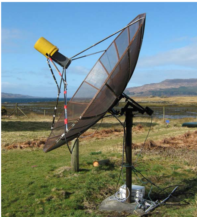
GM4PMK's 3.2 m dish with 1296 feed
