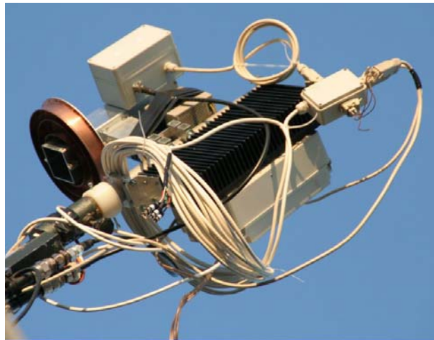
OK1DFC's feed for his 10 m dish and 150 W SSPA used in 13 cm DUBUS contest.
