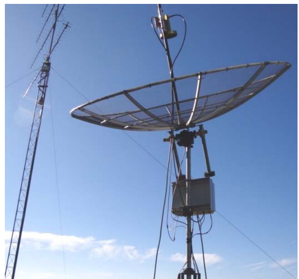
S50C 2.4 m dish used on 13 and 9 cm
