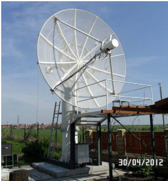
OK1KKD 4 m dish used on 13 cm in DUBUS EME Contest
