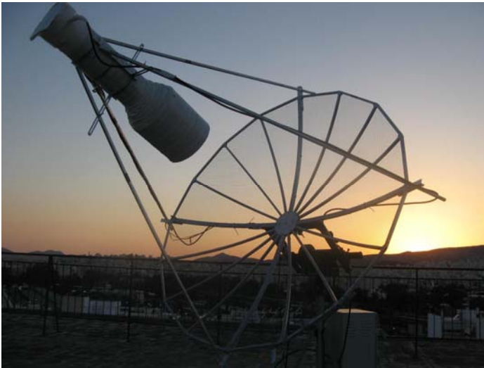
SV1CAL 2 m dish with N2UO feed for 23 cm
