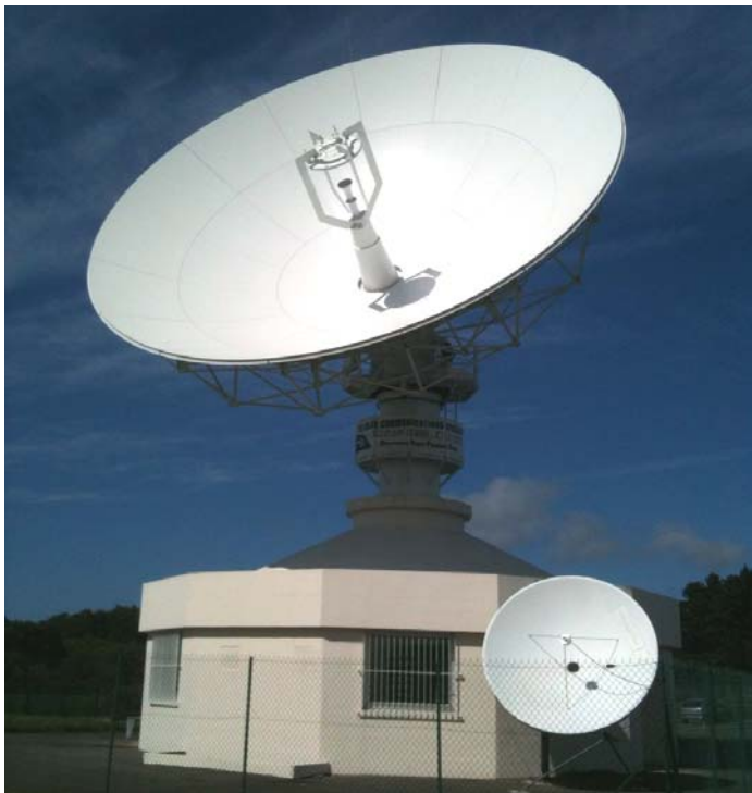
TM9PB 13 m dish used for 6 cm EME tests – see report
