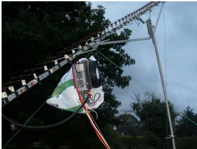
Combination 70/23 cm long yagi used for MN/DJ4TC and /DL2NUD with 1296 150 W SSPA on Jersey and Guernsey Island
