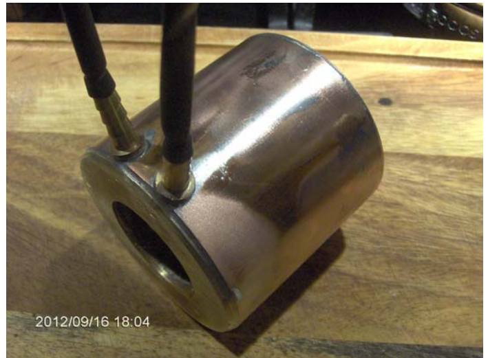
N4PZ's GS35b water cooling jacket.
