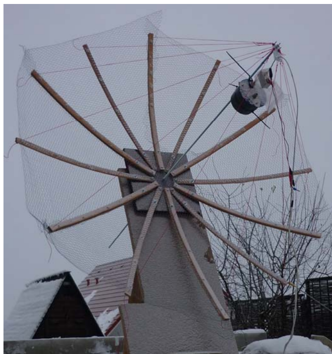
DH5NAH 1.8 m "old bed" stress dish
