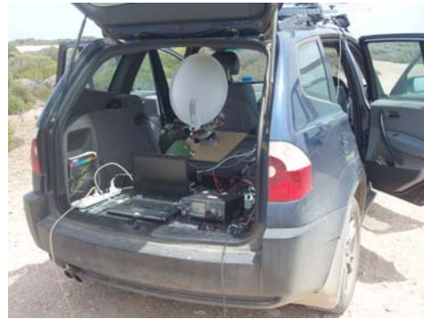
Figure 2: IC-910 and computer set up in the back of car – the small dish is for 24 GHz but was not used (may-be next trip).
