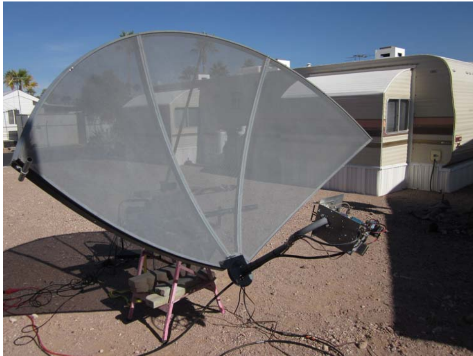
VE4MA's 5' offset dish made from 1/4 10' dish with dual dipole feed for 23 cm
