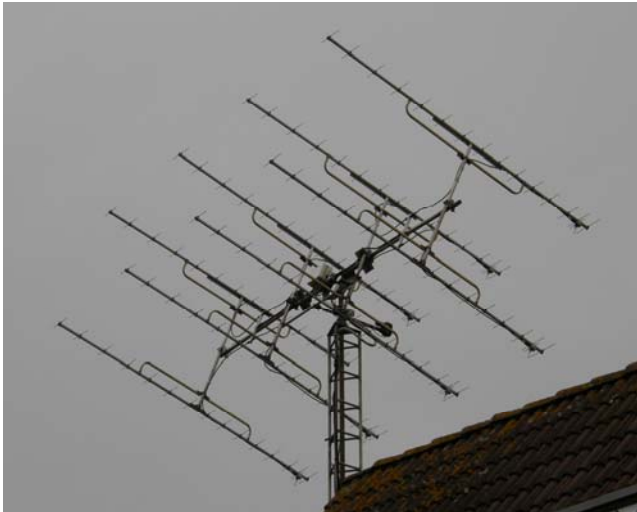
PA0PLY's 8 x DL6WU yagi array
