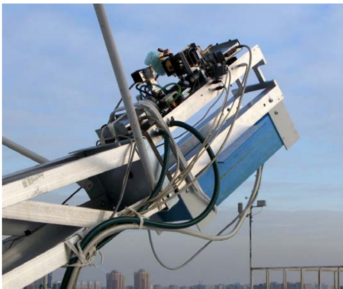
RW3BP's little feed used to receive 77.5 GHz Moon echoes
