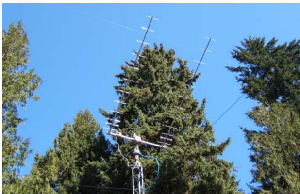
KB7F's 2 x12 el yagi array used with 75 for 70 cm EME
