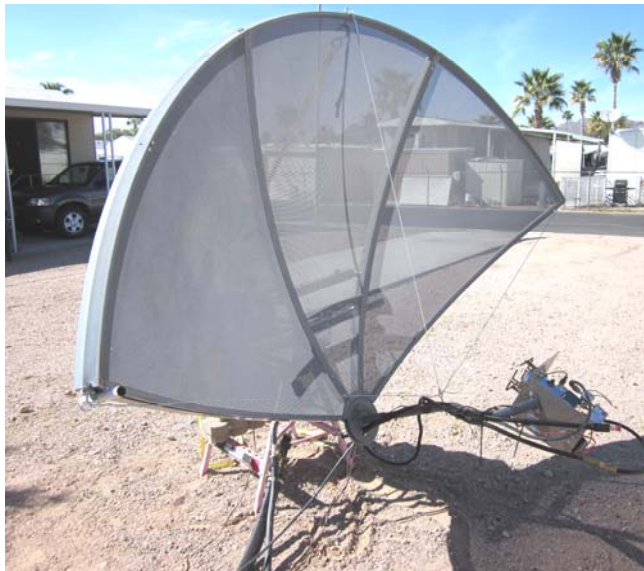
VE4MA/7 5' dish (1/4 of 10' dish fed offset) with 1296 feed
