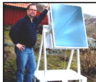
using only a HB horn antenna with a 0.78 m x 0.98 m aperture, a G4DDK VLNA and a TS-2000X transceiver.
