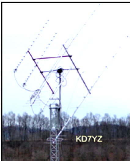
EME array for 2 m (right) and 70 cm (left) - 4 x 18 el 432 LFA yagis with "Splitter Bar" attached to the horizontal H-Frame bar and mounted
