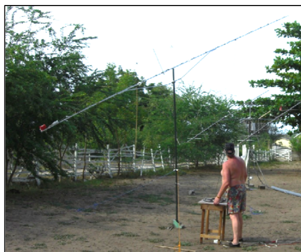
9G5EME used a 23 el yagi and 100 W on 432 to make 23 QSOs
