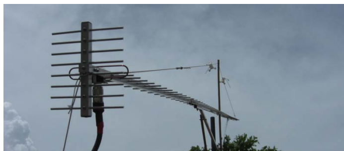
9G5EME's 23 cm 59 el yagi and 100 W made 15 QSOs
