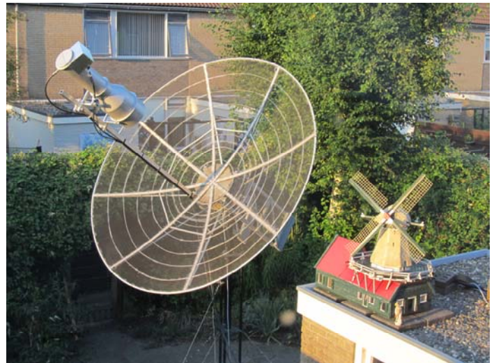
PA3FXB 3 m dish used for 23 cm ISS QSO & EME
