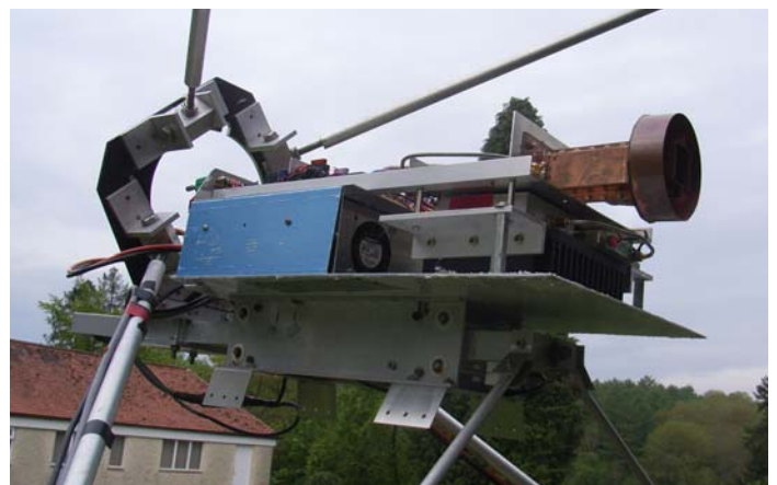
G100RSGB (G4NNS) feed & xverter/SSPA for 6 cm
