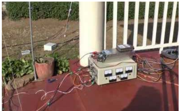
9X0EME's PA connects through a short feed to end of the yagis
