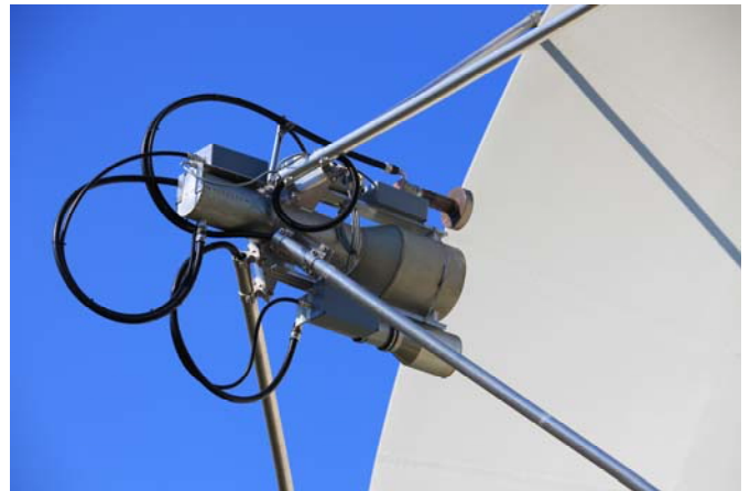
Feeds (23, 13 & 9 cm) mounted offset on new HB9Q 10 m dish
