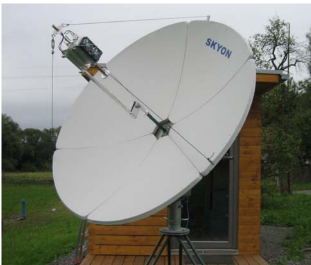
OK2AQ's 3 cm setup consisting of a 1.8 m and 20 W SSPA
