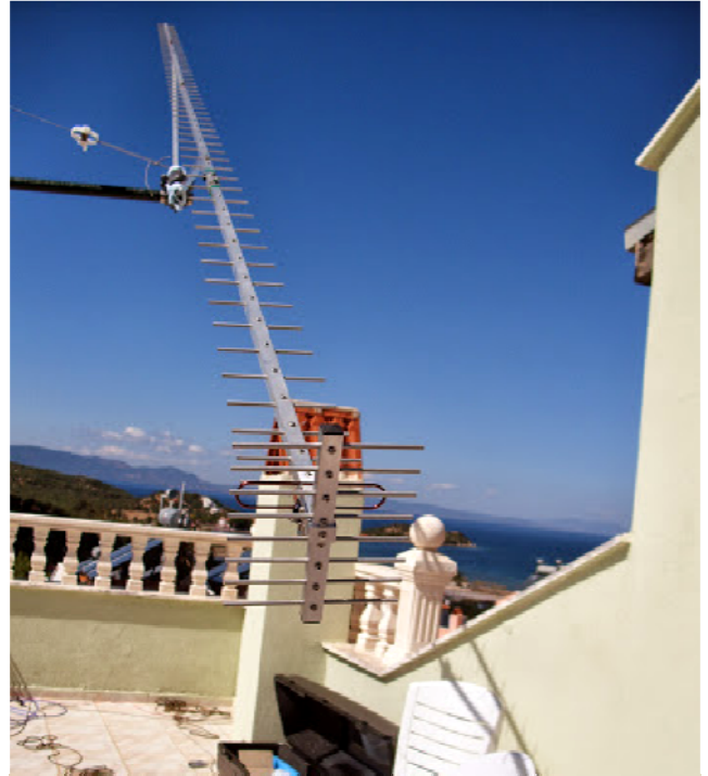
1296 EME from Turkey: TA/PEIL 67 el yagi used on 23 cm
