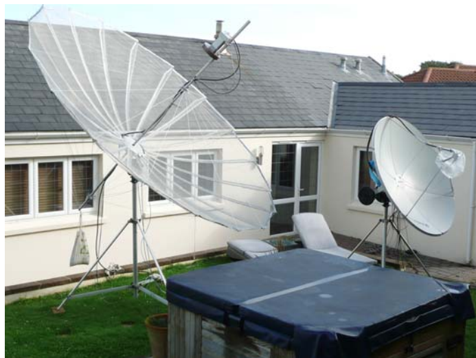
MJ/DL1YMK: stress dish used on 70 – 6 cm & 1.8 m solid on 3 cm
