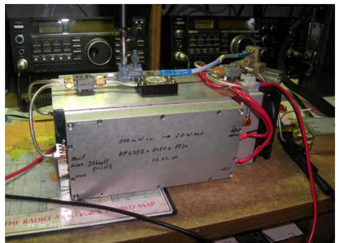
DL1YMK's 40 W 3 cm SSPA during test
