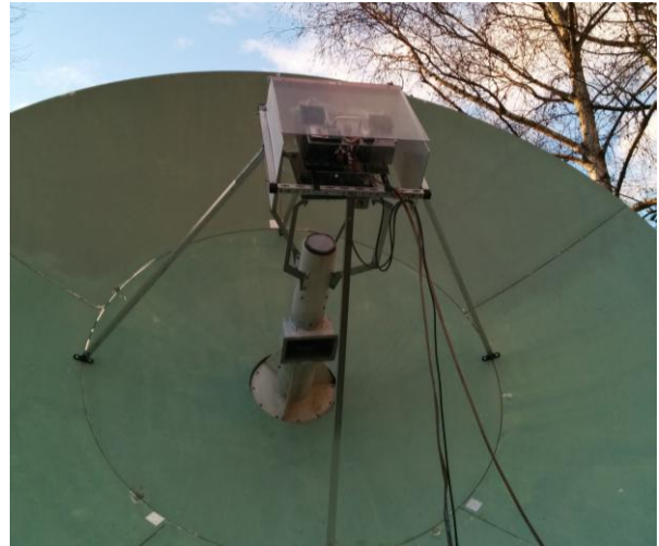
F1PYR 24 GHz feed box and 3.5 m dish – see end of NL
