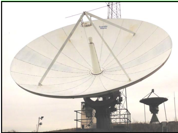
DL0SHF's 10 GHz EME beacon 7.8 m dish
