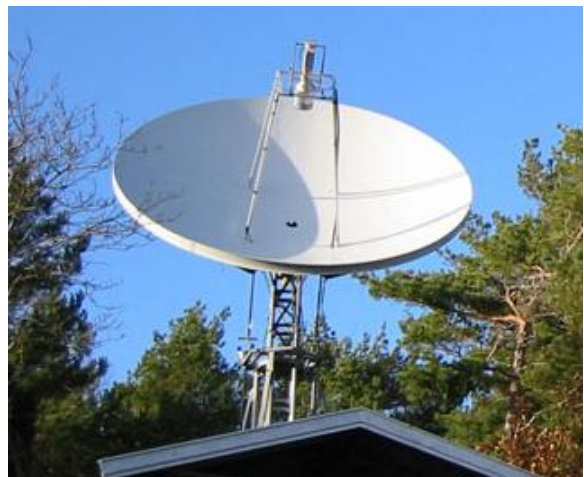
SM6HZF's dish with 1296 feed
