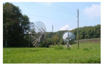
HB9SV's antenna showing big 10 m dish and 10 GHz dish
