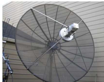
N6OVP's 10' dish with 23 cm feed
