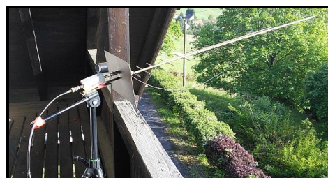
23 cm small antenna EME at DC9UP
