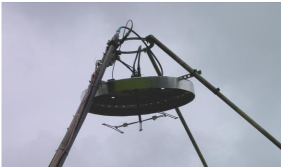
G3LTF's improve 432 feed with baffle
