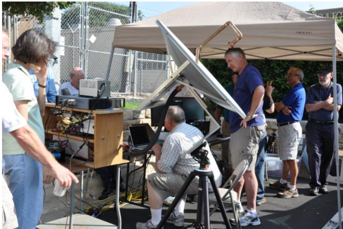
Portable 10 GHz EME demonstration at CSVHF Conference. WA5YWC at controls in QSO with OK1KIR. (Station was built by W5LUA and W5YWC)
