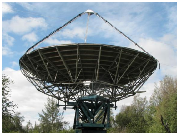
KL6M has his 30' dish back in operation with both coax for low bands and waveguide feed for 6 cm
