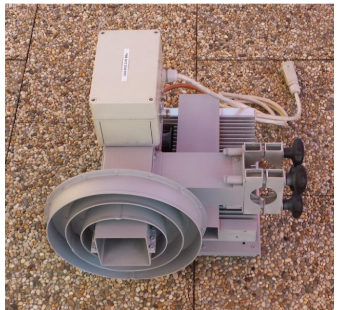
OK1DFC's 13 cm feed with 250 W SSPA and LNA
